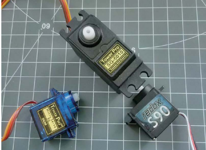
2. Typowe serwa modelarskie: TowerPro Sg90, Redox S90 (9g) i TowerPro SG5010 (36g)
